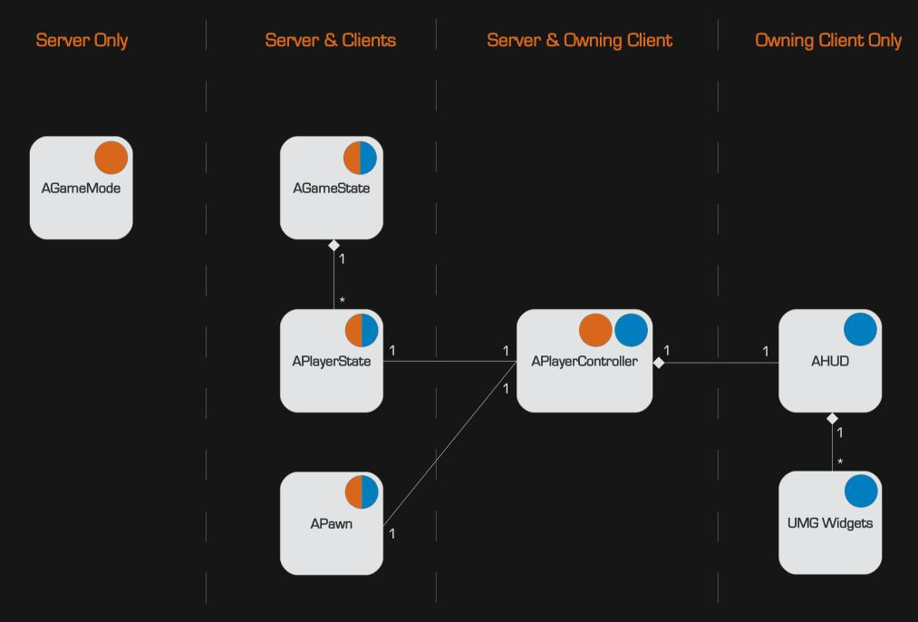
This is how some of the most important classes are laid out in the network framework. (Source 2\*)
